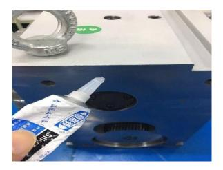
2. After the servo motor installation completed, evenly apply waterproof sealant to the edges of the connecting plate:
