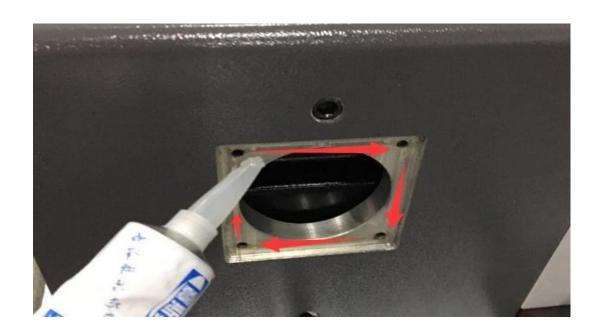
4. After all servo motor accessories are installed, evenly apply waterproof sealant to the mounting surface of motor cover.
